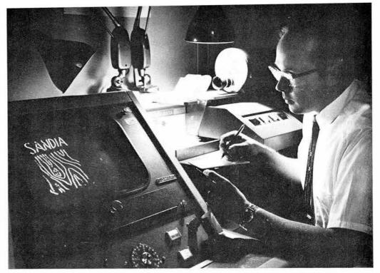
CONTOUR LINES of a terrain map and a handwritten "Sandia" are projected on the Sandia Image Digitizer's monitor screen as R. K. Cover (2565) notes some operations. The Sandiadeveloped system converts illustrations, such as graphs and waveforms, to digits for computer processing.
